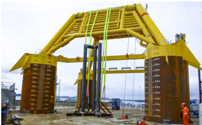
Fabricated Suction anchors with well head template (sea floor protection against unintended damages). Here seafastened for transport to offshore oil-field.
