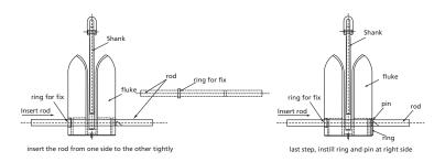
3 – install rod through shank and fluke firmly
