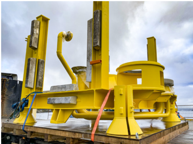
Subsea structure designed and manufactured for up to 25 years in subsea service before pulling up.
