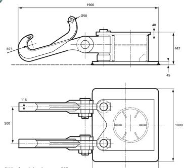
SWL of each hook:60TTest load of each hook:120TCapasity of base:120TSteel:35CrMo + DH36
